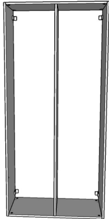
CUIDADO AO FURAR COM A BROCA DE 3MM O PRÉ-FURO NAS LATERAIS PARA NÃO ULTRAPASSAR A ESPESSURA DA PLACA. É APENAS UM PRÉ-FURO CURTO PARA GUIAR E PODER PARAFUSAR OS PARAFUSOS COM MAIOR FACILIDADE.
