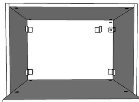
CUIDADO AO FURAR COM A BROCA DE 3MM O PRÉ-FURO NAS LATERAIS PARA NÃO ULTRAPASSAR A ESPESSURA DA PLACA. É APENAS UM PRÉ-FURO CURTO PARA GUIAR E PODER PARAFUSAR OS PARAFUSOS COM MAIOR FACILIDADE.
