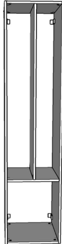
CUIDADO AO FURAR COM A BROCA DE 3MM O PRÉ-FURO NAS LATERAIS PARA NÃO ULTRAPASSAR A ESPESSURA DA PLACA. É APENAS UM PRÉ-FURO CURTO PARA GUIAR E PODER PARAFUSAR OS PARAFUSOS COM MAIOR FACILIDADE.
