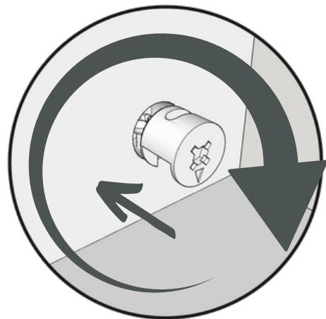
DEPOIS DE ENCAIXADO, COLOQUE O TAMBOR GIROFIX NA BASE E TOPO E GIRE COM A CHAVE PHILLIPS PARA DAR APERTO.
