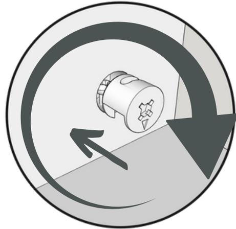
DEPOIS DE ENCAIXADO, COLOQUE O TAMBOR GIROFIX NA BASE E TOPO E GIRE COM A CHAVE PHILLIPS PARA DAR APERTO.
